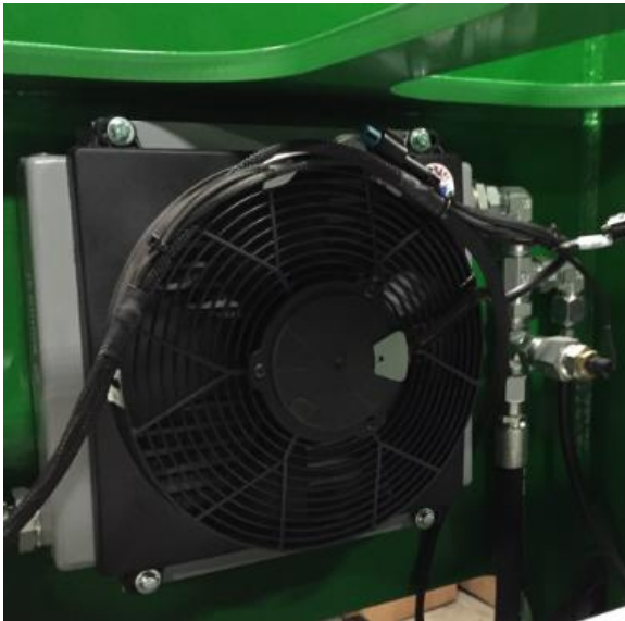
ELECTRIC, HYDROLOGIC OIL COOLER- On/ Auto switch located on the main console. Turns on at 135 degrees when set in auto mode.
