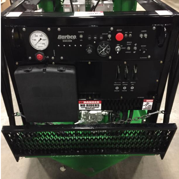
FOLD DOWN PLATFORM- Offers a place to stand on during maintenance procedures.
