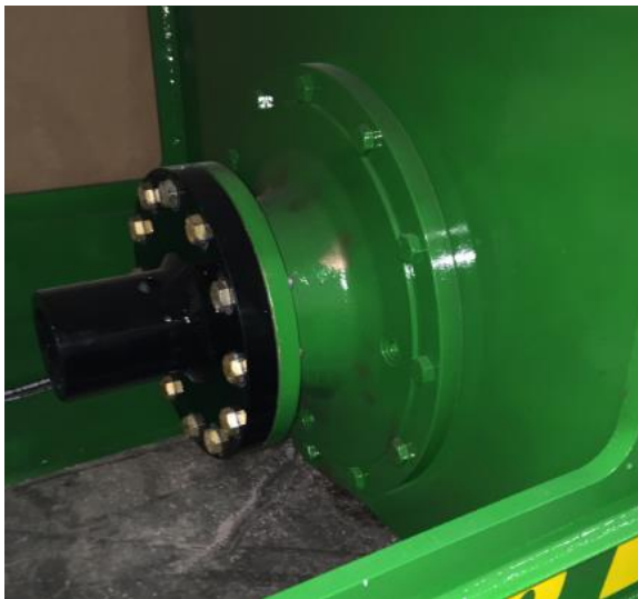
FRONT DRIVE- Hex ID final drive and gearbox assembly.
