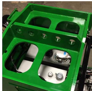
MAIN LIFT POINT BAR- Adjustable lift points to balance the machine
