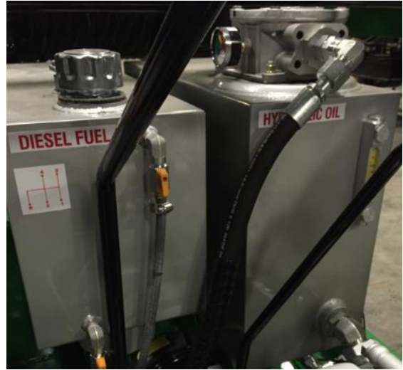
TANKS- Hydraulic and Diesel fuel tanks located under the main lift point bar.
