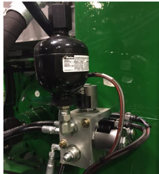
CLUTCH VALVE- Disengages the clutch upon starting the engine. Keeps the operator from climbing on the unit to declutch if the engine stalls.
